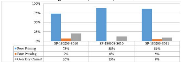
Fig 7. Data of the Rejected Bonding Accelerator LS Shoe June - August 2018 (Customer Return)
