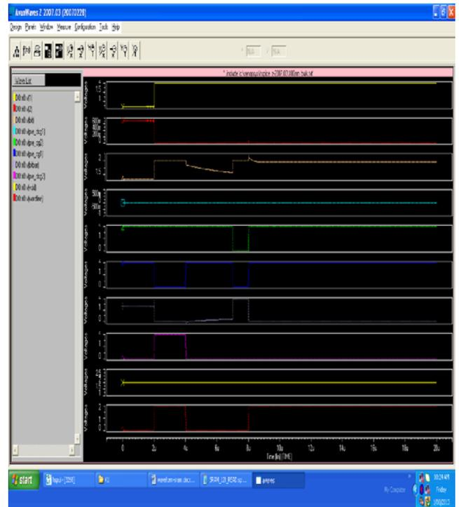
Figure 5: READ Operation - 6T SRAM
