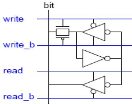
Figure 3: Structure of 12 T SRAM
