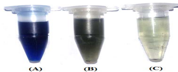
Fig.7. Decolorization of (A) acid blue 25 dye in the presence of the complex as a heterogenous catalyst and H 2 O 2 after 10 min (B) and 50 min (C).
