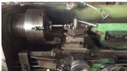
Figure 4 Center drilling of workpiece
