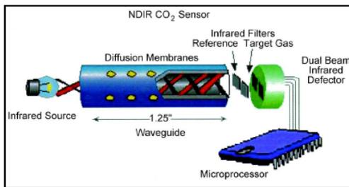
**Fig.3. Non-dispersive infrared detection (NDIR) CO<sub>2</sub>**
