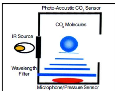
**Fig.4. Photo-acoustic CO<sub>2</sub> Sensor/4**
