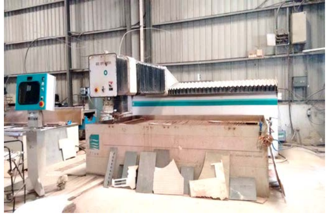
Fig.1 CNC Abrasive water jet Machine Setup
