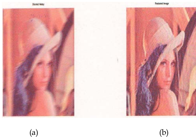
Fig 4: Lucy Richardson results where a is the Blurred Noisy image with SNR -20\text{dB} , b is Restored image with (MSE=440, PSNR=21.678, NumIt=20)
