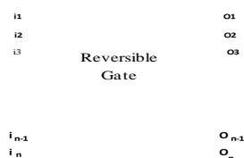
Figure1: A reversible gate with n-inputs and n-outputs is called  $n \times n$  gate.
