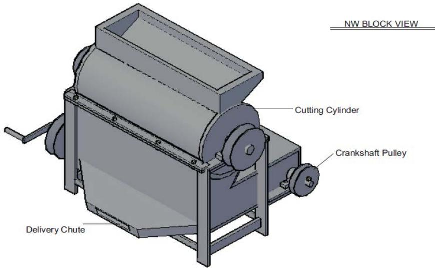
Fig. 1: Isometric drawing of orange juice extractor
