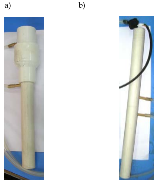
Fig. 5: a) Pneumotachometer with change in tube diameter b) Pneumotachometer without change in tube diameter
