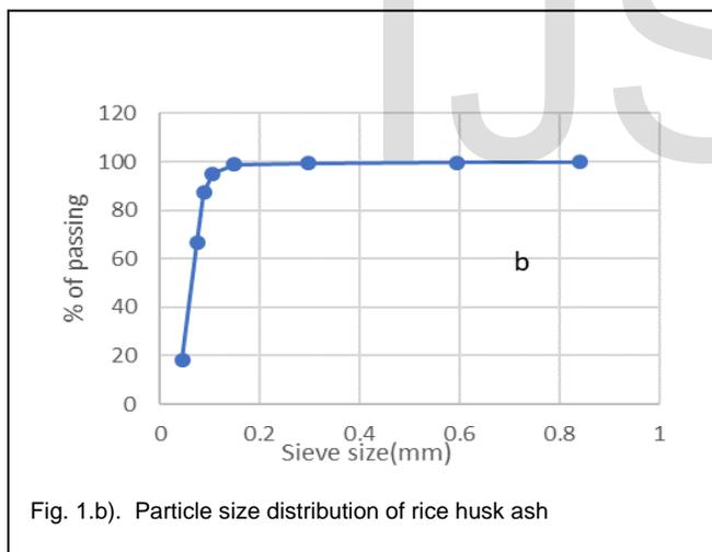
Fig. 1.b). Particle size distribution of rice husk ash
