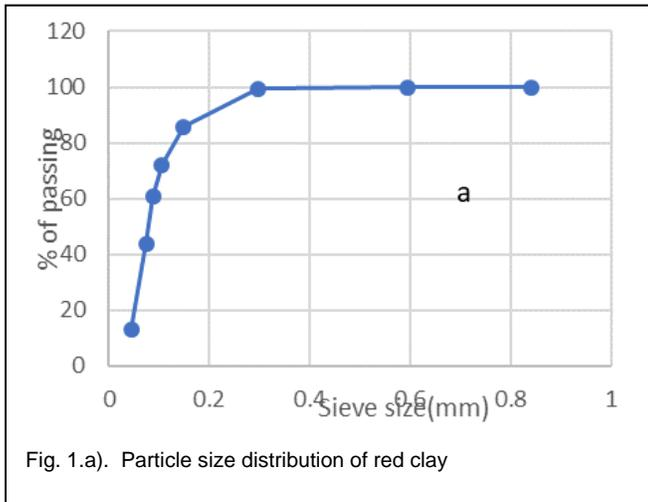
Fig. 1.a). Particle size distribution of red clay
