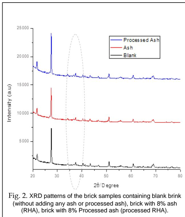
Fig. 2. XRD patterns of the brick samples containing blank brick (without adding any ash or processed ash), brick with 8% ash (RHA), brick with 8% Processed ash (processed RHA).
