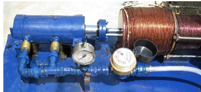
Fig. 7: Electromagnetic oscillator coupled to double-acting reciprocating pump
