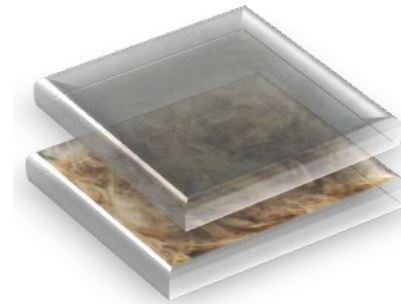
(Betel nut fibers were sandwiched between two pp sheets according to different wt. %)
