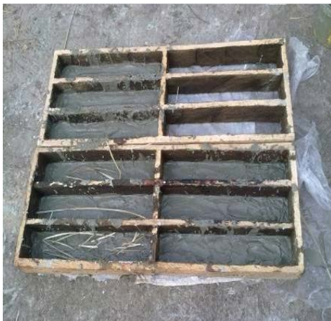
Fig. 3. SIFCON Beam Sample Preparation
