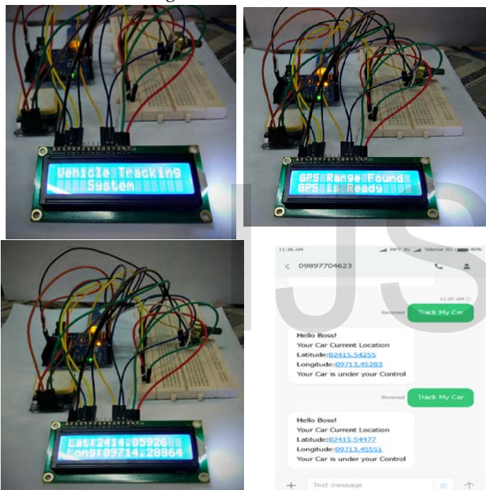
Figure 12. Overall Test Results
