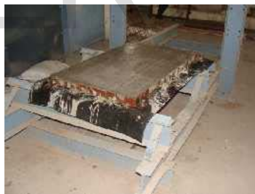
Fig.1 Rectangular steel frame with flexible PU membrane for casting the pre mould
