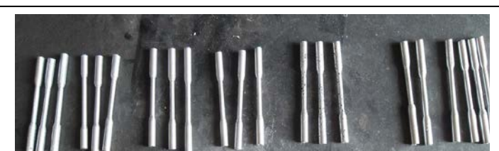
Fig. 1. Tensile specimens according to ASTM B557M specifications
