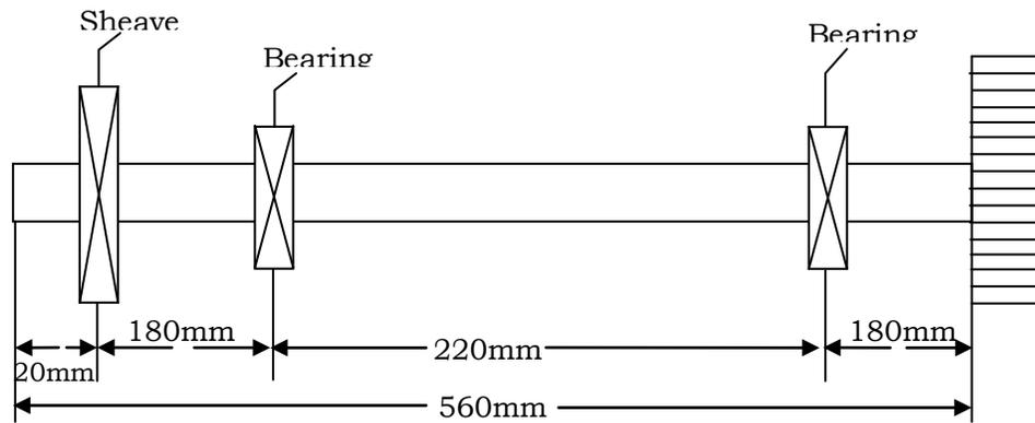
**Fig 2: Axial, torsion and bending loads on the shaft**
