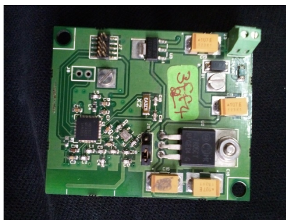
Figure-4: Beacon internal circuits
