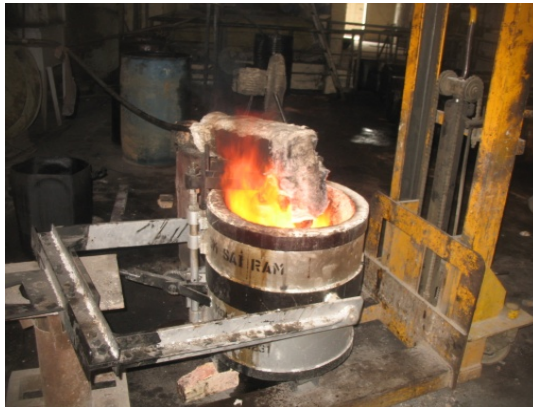
Fig. 3: Oil Nozzle Preheat Current)
