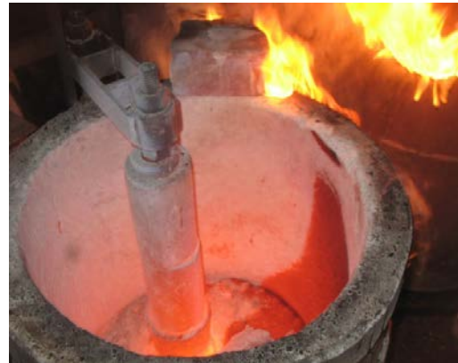
Fig 4: Heated Ceramic and Stopper Rod
