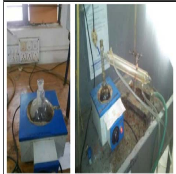
Fig.4 - simple dehydration and distillation
