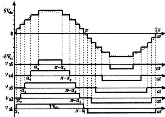
Fig. 2. Output voltage waveform of an 11-level cascaded H-bridge multilevel converter using fundamental frequency switching scheme.
