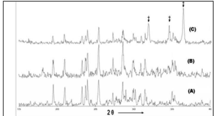
Figure 1: XRD patterns of (A) SCaP-750 (blank), (B) ZnO/SCaP(150) and (C) ZnO/SCaP(400)
