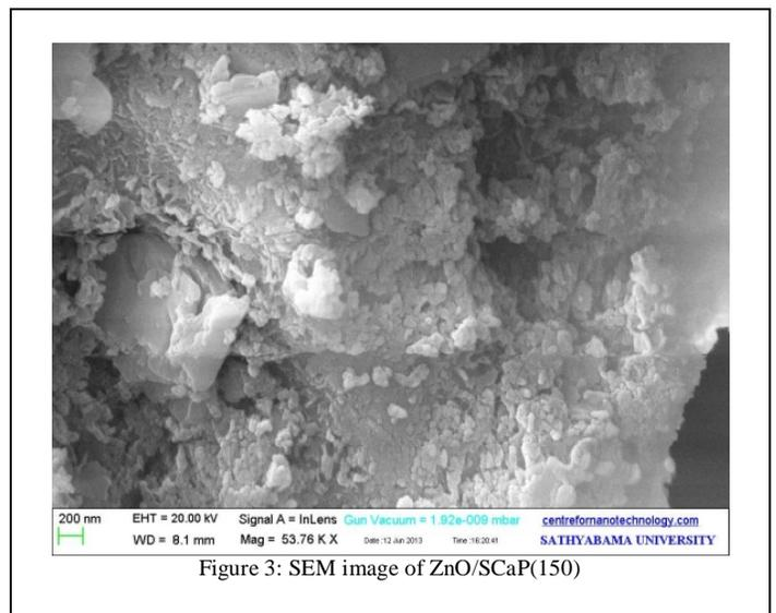
Figure 3: SEM image of ZnO/SCaP(150)
