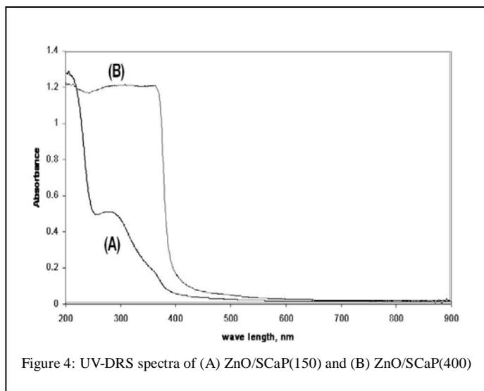
Figure 4: UV-DRS spectra of (A) ZnO/SCaP(150) and (B) ZnO/SCaP(400)
