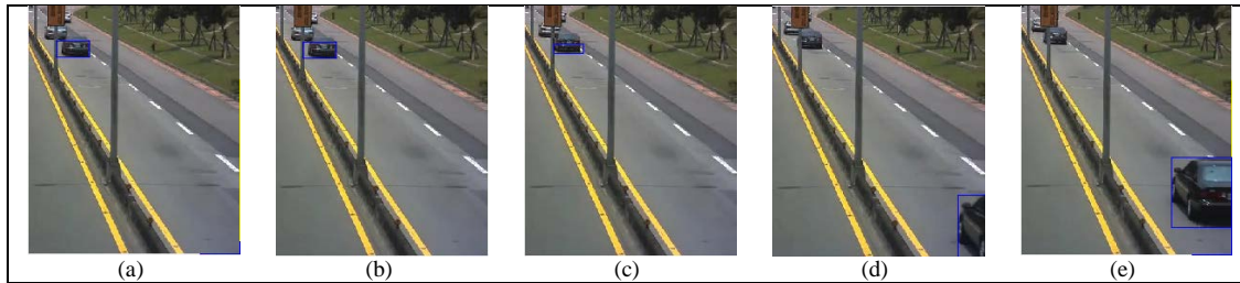
Fig. 4. Detection and tracking of vehicle by kalman filter for an image sequence. Please note that the given sequence is intermediate samples and not temporally interlinked with each other.
